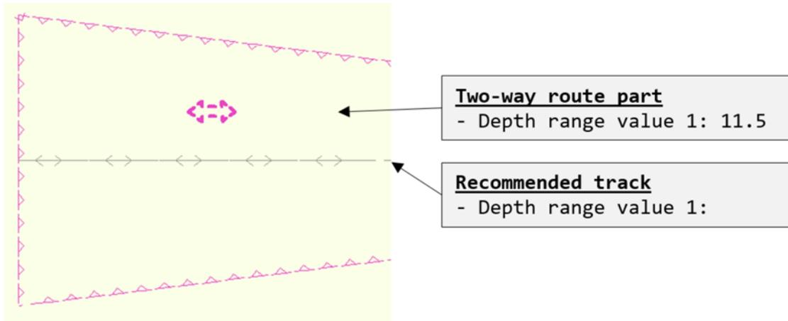
Navigation line and fairway area on an ENC chart. The safe clearance depth of the fairway area is stated as the Depth range value 1 (DRVAL1). (The presentation method on an ECDIS device may differ from the example.)
